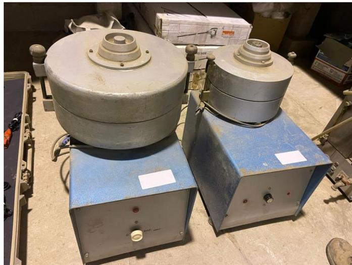
**DETALLE: 2 UN MÁQUINAS DE PRUEBA DE ASFALTO CENTRÍFUGO.**
