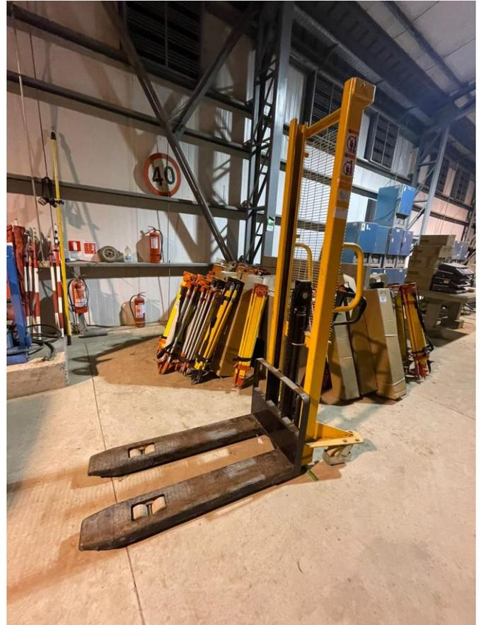
**DETALLE: 1 TRANSPALETA HIDRÁULICA 1000 KG**
