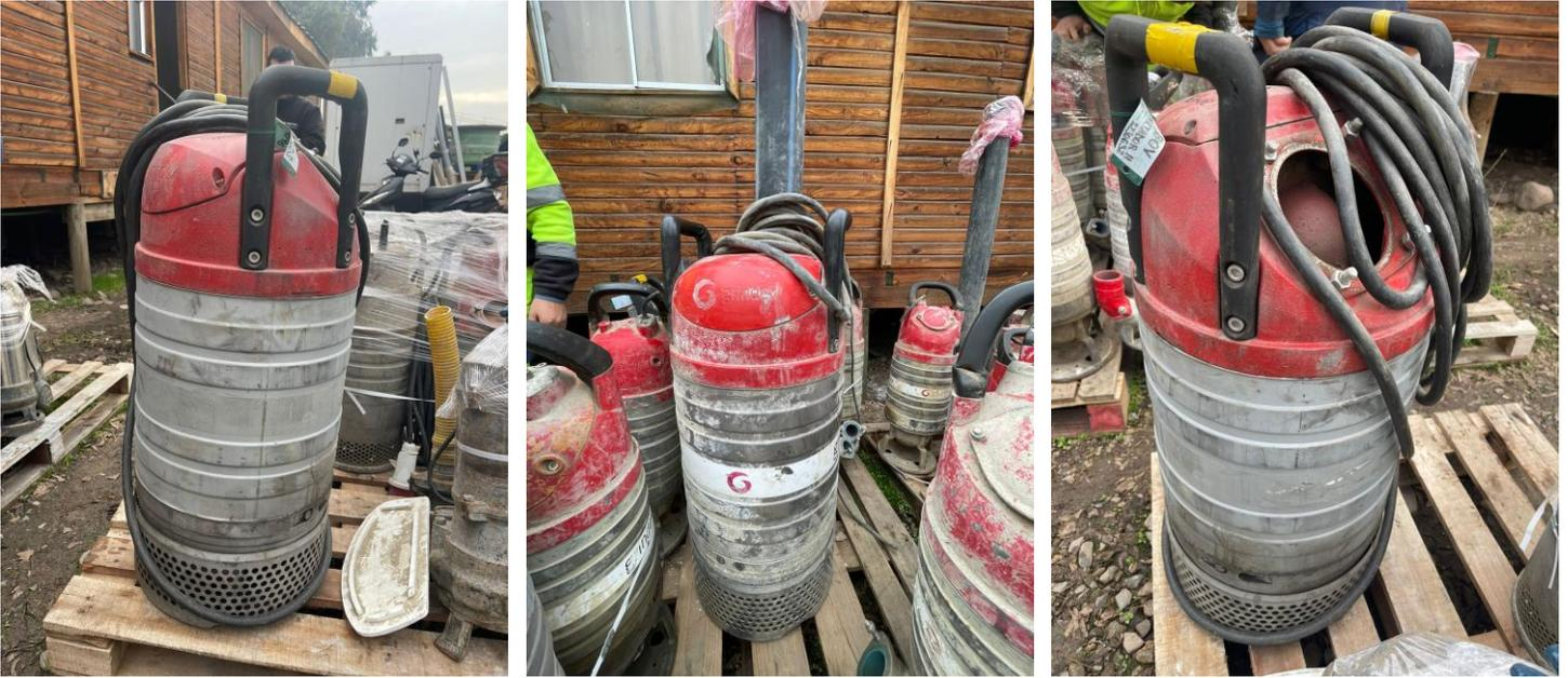
**DETALLE: 2 UN BOMBAS SUMERGIBLES MARCA GRINDEX DE 4.**
