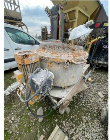
**DETALLE: 7 UN. LECHADORAS PARA HORMIGÓN CON TABLERO Y MOTOR**
